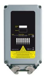
M880 L receiver for its compact size and amazing versatility is the ideal receiver for most of the on/off application in AC and DC as well as for standard proportional applications DC such as hydraulics cranes. Its installation on the machine will be simple and unobtrusive.
